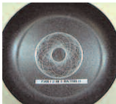
Coating "A" earns a "0" rating (total failure) after Whitford's Gyrograph Test.
