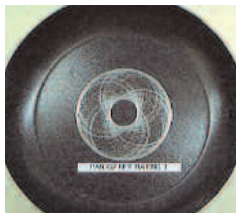
Coating "B" earns a rating of "1" after the same test and same # of cycles.
