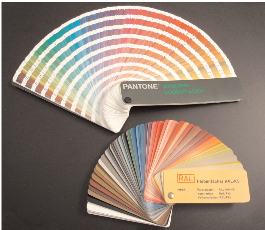
Pantone and RAL are the two leading international standards for color matching. Providing a specific color from one or the other goes a long way toward simplifying color matches for cookware that Whitford does in our Laboratory. A request for "blue" doesn't help. "Pantone 286 blue" does.
