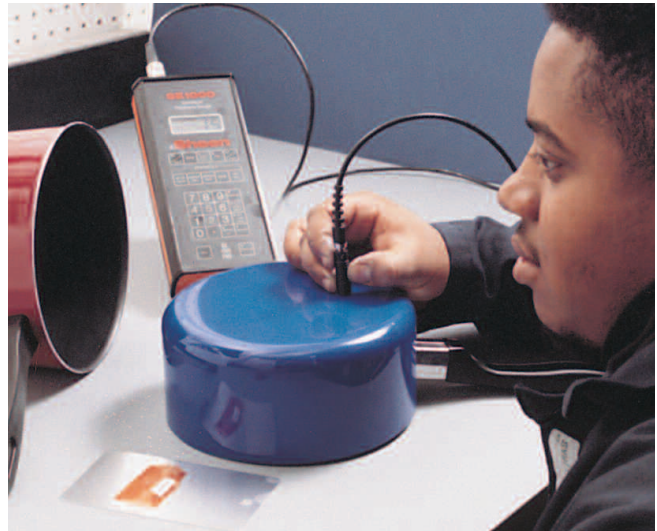
Measuring dry-film thickness (Whitford Test Method 114A) is a key part of the QCP testing program. If specified film thicknesses are not met, the coating will not perform up to expectations.
