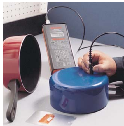
Whitford technician tests coating thickness as part of the QCP.
