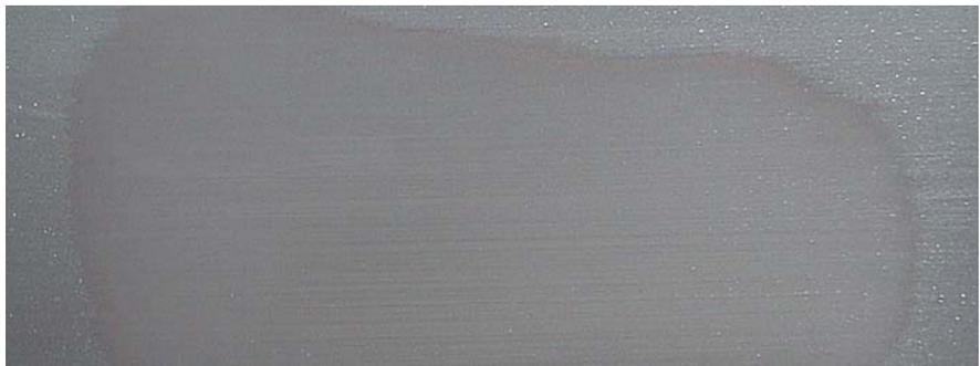
New Eclipse after more than 200,000 cycles on the RAT. The coating has been polished, but has not worn through and continues to perform normally.
