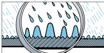
Molten stainless steel is applied to the surface, building up a matrix of “peaks” and “valleys”.
