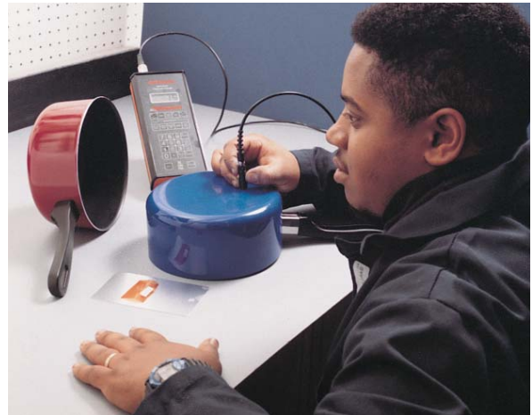
Whitford's Test Method 114A (dry-film-thickness test) is fast and reliable, but does require having the right electronic equipment.
