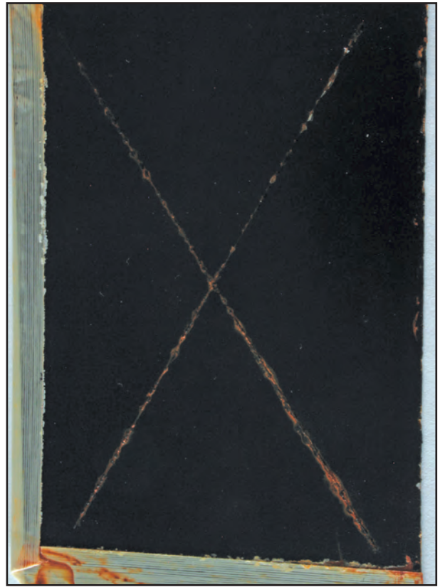
Skandia Xtreme Plus with a DFT of 7-9 microns after the same salt spray test. No migration evident, corrosion shows only where the test panel is scored. After 5 tape pulls, no coating is removed.
