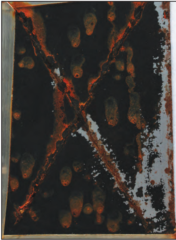
Conventional bakeware coating with a DFT of 6-8 microns after 350 hours Hot Salt Spray (ASTM B117). Heavy migration evident, serious corrosion results. A standard tape pull removes coating.
