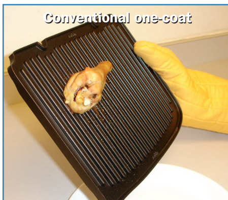
In the Grilled-Chicken test, the first piece stuck to the grill with the conventional one-coat. Rated a "fail".
