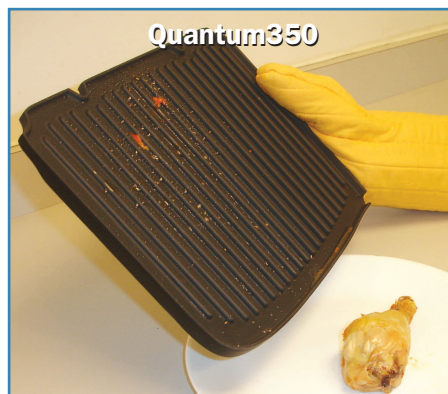
The grilled chicken on the grill coated with Quantum350 did not stick, but released and fell off the surface. A perfect "pass".
