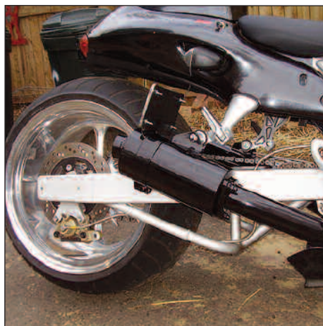
Xylan extremely high-heat powder coatings are designed for use on mufflers, exhaust pipes and engine gaskets for vehicular applications.
