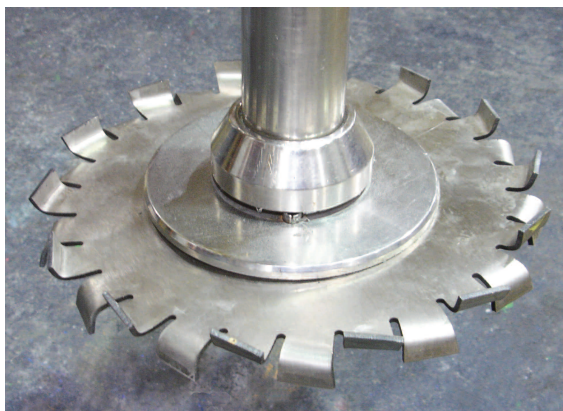
A toothed impeller for the proper mixing of the Fusion products.
