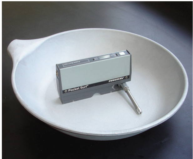
A Profilometer, shown here, provides an accurate measure of surface roughness.
