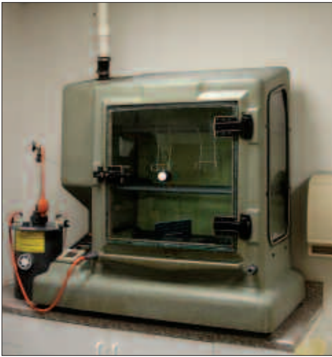
Whitford keeps Kesternich cabinets running virtually all the time at several of its research laboratories around the world.
