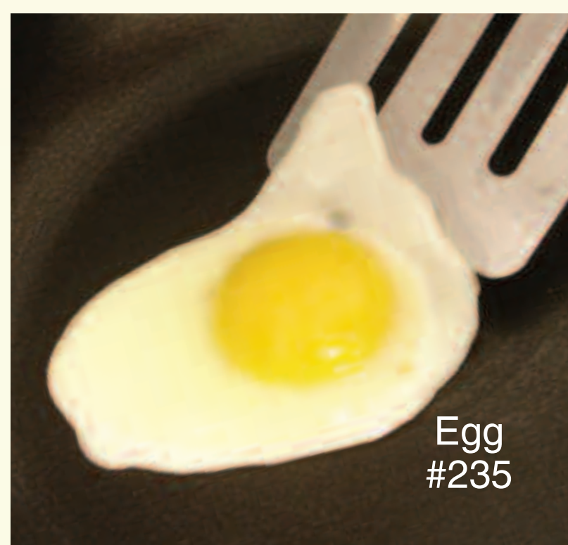
The Dry-Egg test on the new Eterna™ coating at Whitford's laboratory. All these eggs continued to lift easily off the dry surface of the pan, including #350, at which point the test was stopped.
