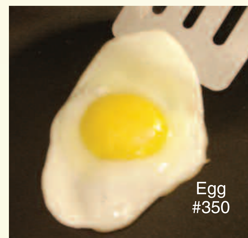
The Dry-Egg test on the new Eterna™ coating at Whitford's laboratory. All these eggs continued to lift easily off the dry surface of the pan, including #350, at which point the test was stopped.
